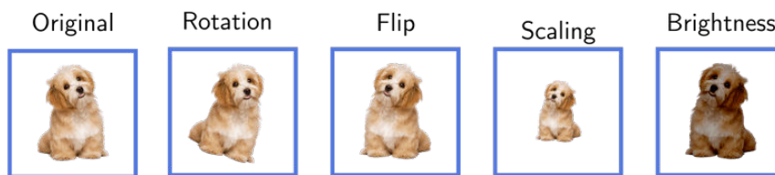
Figure 32: Examples of Data augmentation. The original data point is multiplied without the need to go out in the world and collect more unique data points.
